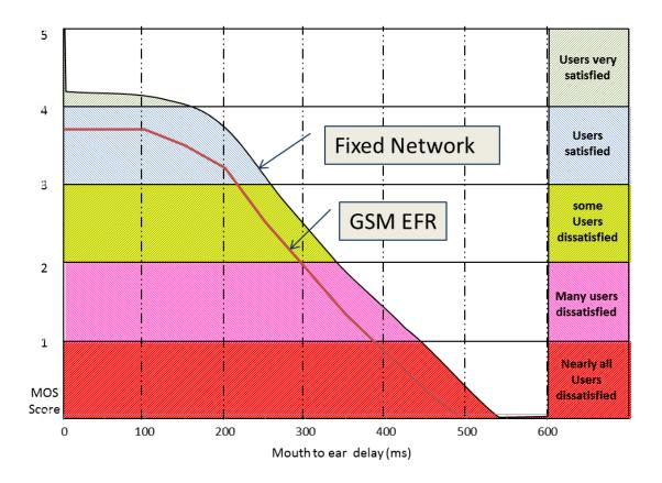
The Mean Opinion Score (MOS) defining the perceived quality is 4.3 for fixed Telephony. The score for a GSM network relying on terrestrial backhaul is between 2.9 and 4.1. In case of GSM backhaul by satellite the MOS is between 1 and 2.
