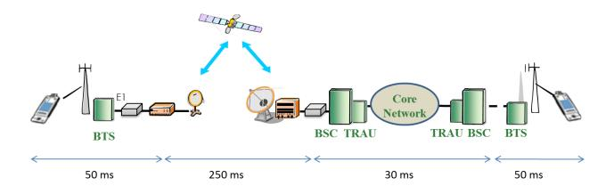
In the case of local communication between 2 GSM users connected to a BTS backhauled by satellite as illustrated hereafter, the voice traffic is going through the satellite to the core network and back again adding an extra propagation delay of 250 ms for a total of 630 ms. As we will see later, this level of latency has a significant impact on the quality of service as perceived by the end-users.
