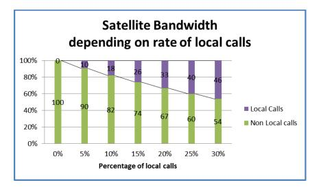
The above figure shows that a significant rate of local calls can have a big impact on the cost of satellite bandwidth.
