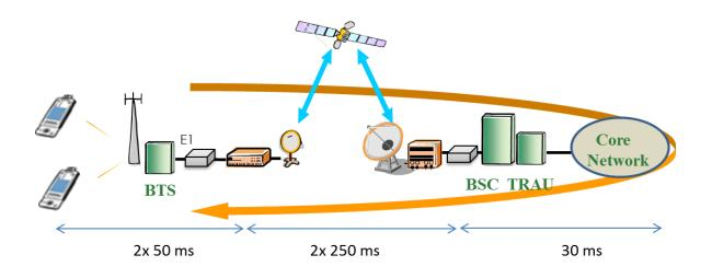
As shown below, the Local Switching solution allows for reducing the one way transit delay for local calls in the range of 100 ms.
