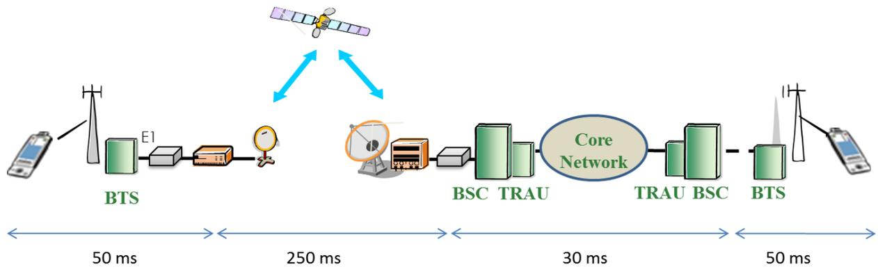
In the case of local communication between 2 GSM users connected to a BTS backhauled by satellite as illustrated hereafter, the voice traffic is going through the satellite to the core network and back again adding an extra propagation delay of 250 ms for a total of 630 ms. As we will see later, this level of latency has a significant impact on the quality of service as perceived by the end-users.
