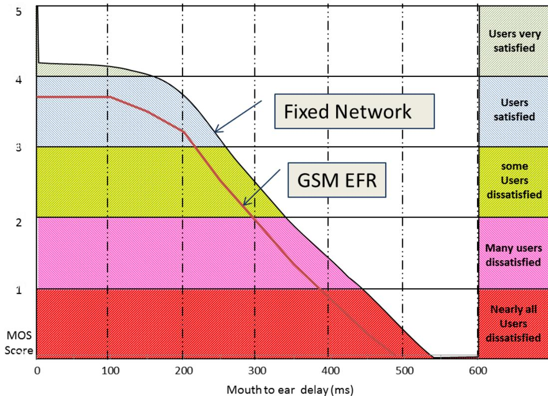
The Mean Opinion Score (MOS) defining the perceived quality is 4.3 for fixed Telephony. The score for a GSM network relying on terrestrial backhaul is between 2.9 and 4.1. In case of GSM backhaul by satellite the MOS is between 1 and 2.
