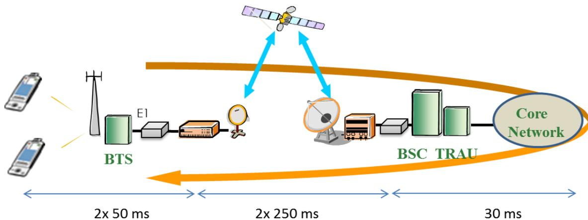
As shown below, the Local Switching solution allows for reducing the one way transit delay for local calls in the range of 100 ms.
