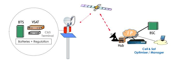
The system is composed by a small embedded electronics (Cell & Sat Terminal, CST) at the site and a central server (Cell & Sat Optimiser and Manager, CSO / CSM). The CST interfaces with the solar charge controller, the BTS and the VSAT. It handles real-time traffic analysis and communicates with the CSO through a secured IP connection. The CSO/CSM hosts powerful databases for system control, optimisation of transmission resources, energy savings mechanisms and statistics.
